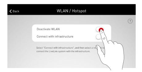
The deactivation in this pop-up must be confirmed. The WLAN switches off after 10 minutes.
