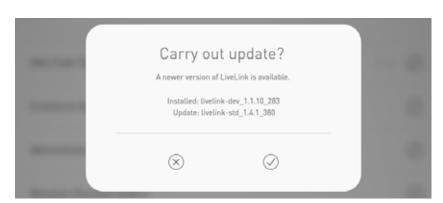
Upon confirmation, the firmware is uploaded to and subsequently installed on the control device ("LiveLink flashing").
