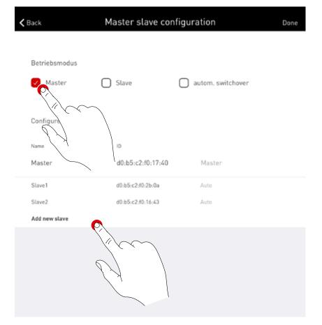
After actuating "Add new slave" a selection box is displayed with all available slave control units. The list only shows control units already connected with the master via WLAN and configured with slave operating mode or autom. switchover.
