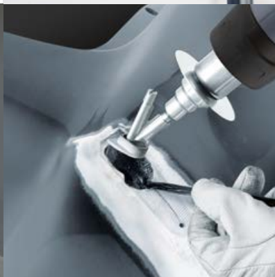
▲ Repairing bumpers HG 2320 E
