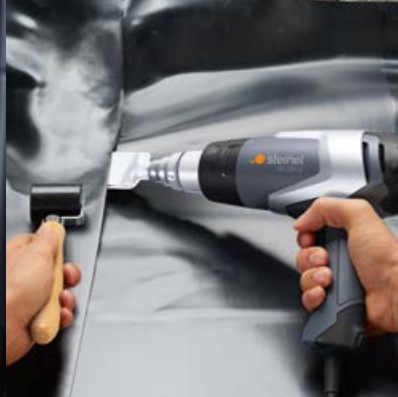
▲ Welding pond liner HG 2320 E
