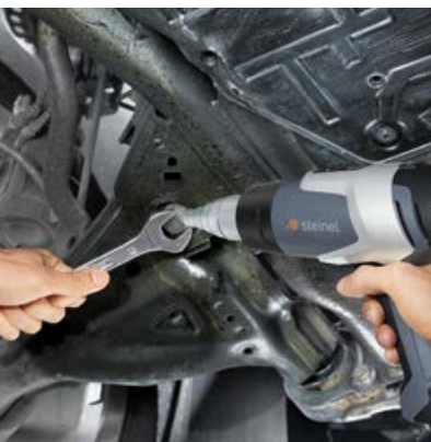
▼ Loosening bolts HG 2320 E
