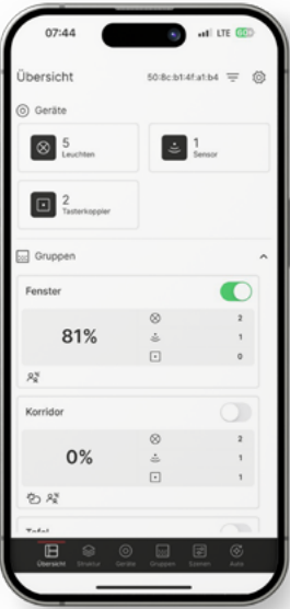
LiveLink LAN DR • DALI-2 APC max. 64 participants • Commissioning via WiFi and app • Connection to higher-level systems via MQTT EAN 4007841 055455
