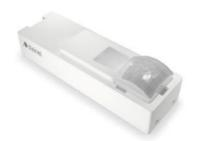
Small. Flat. Compact. Inconspicuous presence detector. 360° passive infrared sensor IR with a presence range of 4 x 4m (presence and radial) or 6 x 6m (tangential). With patented multisegment pyrosensor lens.
